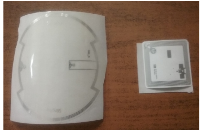
Stingray circular tag for discs (left) and inverted square blocklite tag (right)
